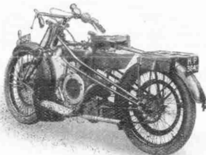
The McKechnie Motor-cycle in its final form fitted with a 5/7 H.P. Coventry-Victor engine.
