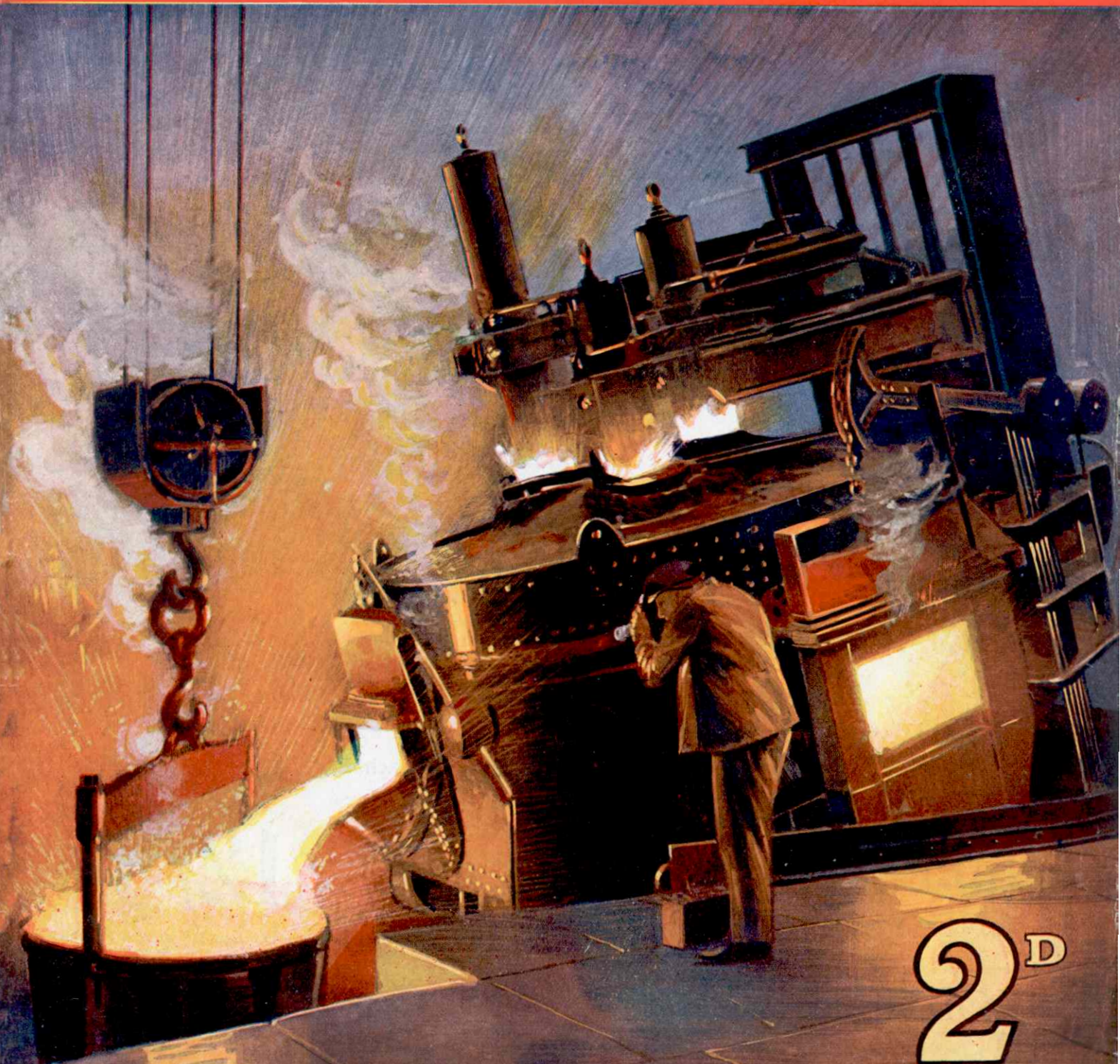
TAPPING AN ELECTRIC FURNACE
