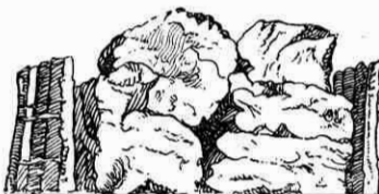
Fig. 1. Method of Constructing Early Breakwater*
