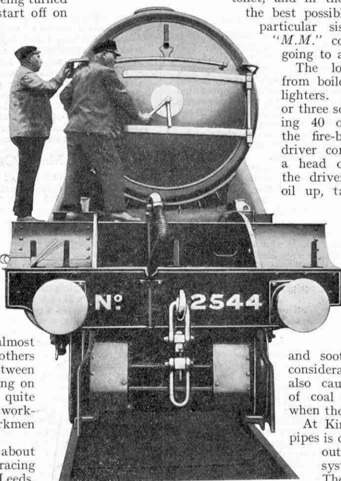
Courtesy] [L.N.E.R.] The Driver screws home the fastener of the smoke-box cover (L.N.E.R. No. 2544 "Lemberg.") If this is not fastened tightly, the engine loses efficiency
