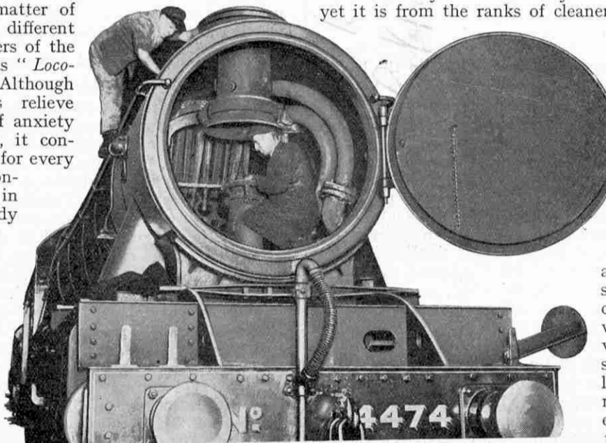
Cleaning the inside of the smoke-box of L.N.E.R. No. 4474, " Victor Wild "
