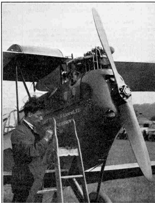
Photo] The nose of the D.H. "Moth" used by the Lancashire Aero. Club at Woodford Aerodrome, showing the simple design of the modern light aeroplane, which is used by many light aeroplane clubs [E. Wilson
