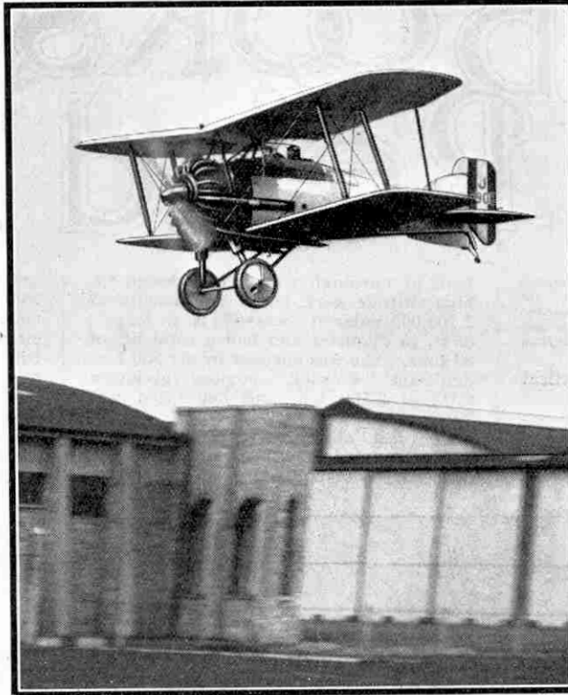
Courtesy] This snap of a Gloster "Gamecock" clearly shows the Bristol Jupiter engine
