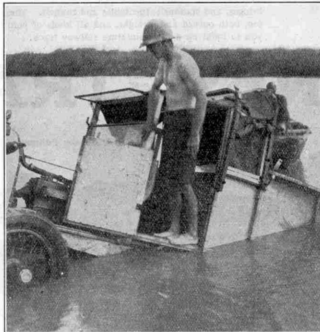
Our two illustrations show the submerged cars, with electrical equipment and carburetters removed being dragged across rivers by natives
