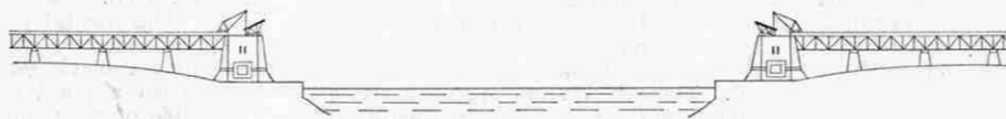
The completion of the approach spans. Staging for Main Span "creeper cranes" being erected on north and south sides by 25-ton cranes
