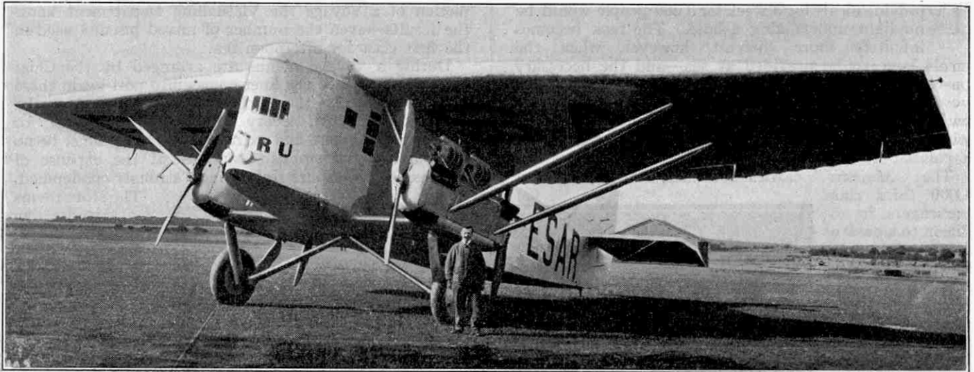
The "Jabiru," fitted with two engines and thickened wings
