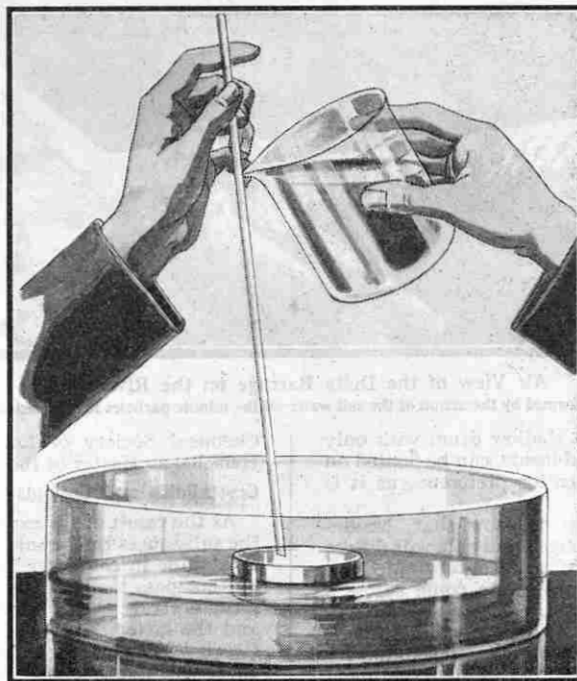
Fig. 1. How the layer of water is added to the blue vitriol solution without mixing. Pouring down the glass rod prevents splashing
