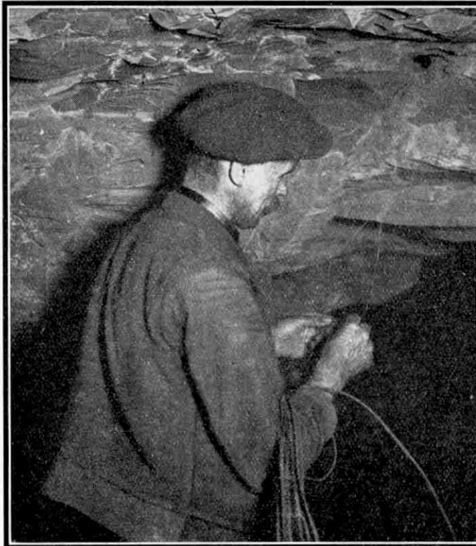
Deputy connecting up the wires from his pocket battery with explosive
