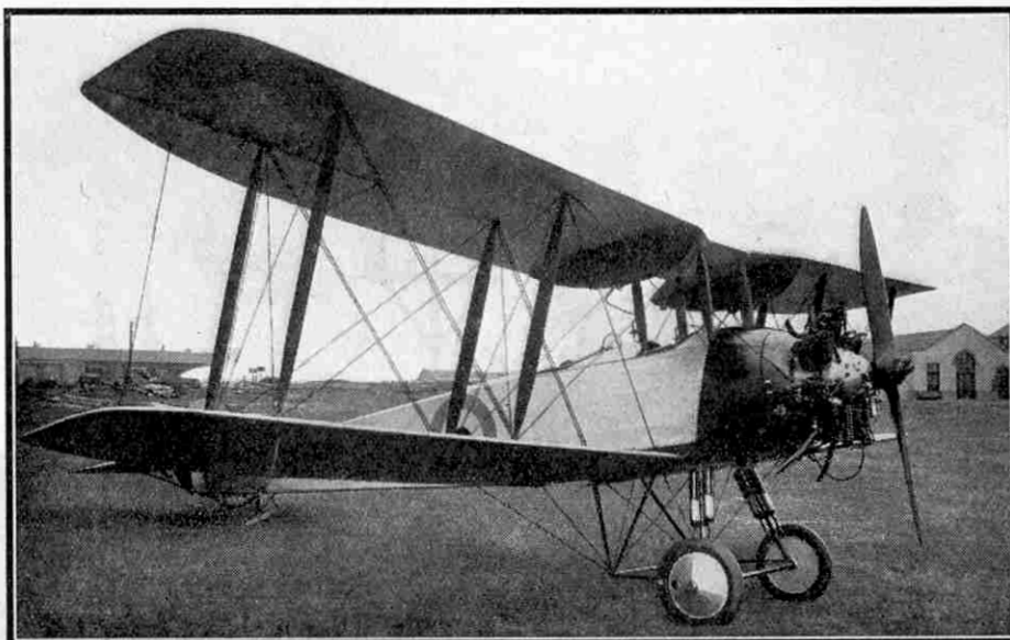
An Avro 504 N, fitted with a 180 h.p. Siddeley Lynx Engine
