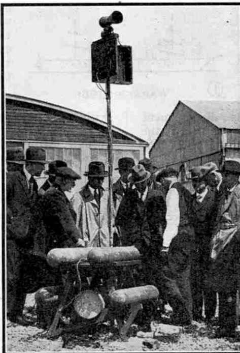
The Directional Fog Signal, an apparatus by which a blindfolded boy steered a ship into harbour
