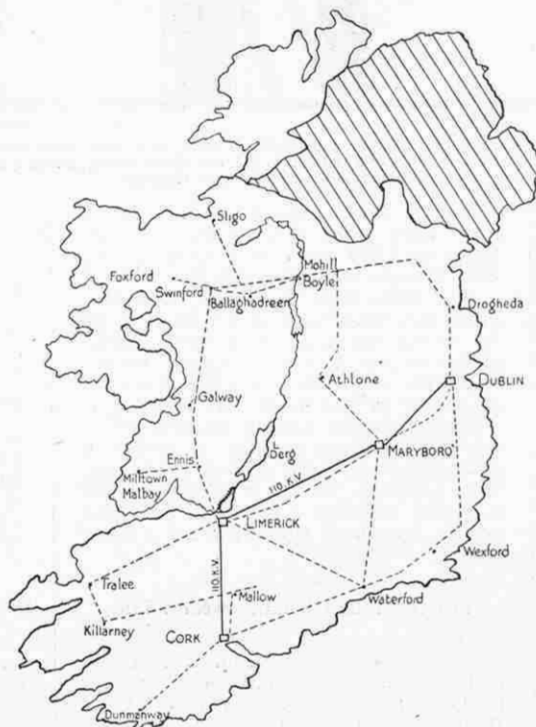
Map showing the main transmission lines of the Shannon Power Distribution Scheme
