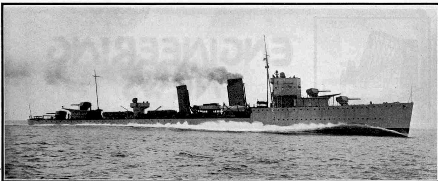
H.M.S. "Amazon," Britain's largest and fastest post-war destroyer, built by John I. Thornycroft & Co. Ltd. at Southampton in 1927. This vessel is 311 ft. 9 in. in length, has a displacement of 1,330 tons and a speed of 37.96 knots
