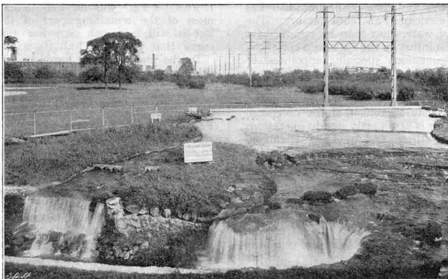
A miniature Niagara! This view of the scale model referred to in the article illustrates a possible method of restoring the full effect of the Horseshoe Fall by placing artificial islands above the crest
