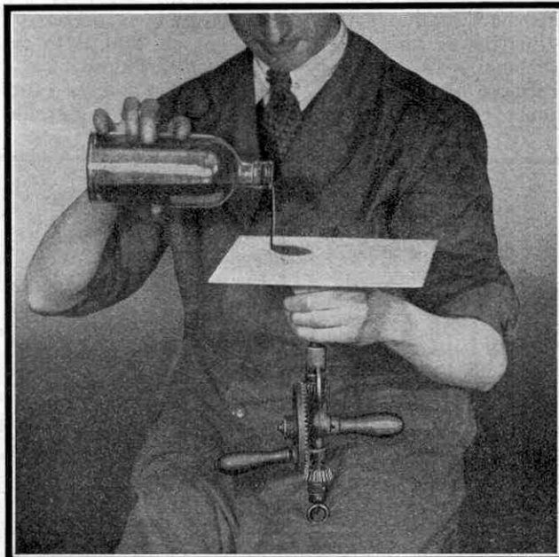
Pouring sensitised fish glue on a copper plate that is to be made into a printing block
