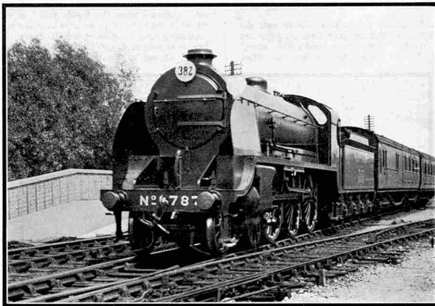
Southern Railway "King Arthur" class Locomotive No. E.787, "Sir Menadeuke" leaving Southampton West Station. This Locomotive was one of the first of the type to be fitted with Smoke Deflectors
