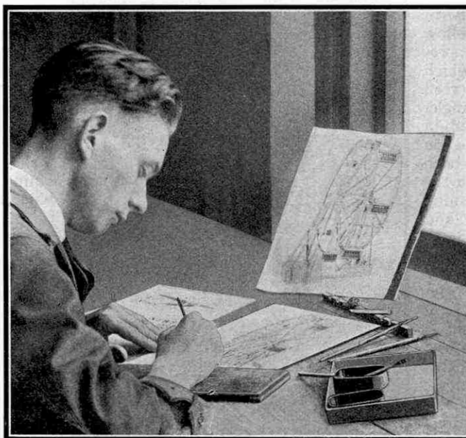
Half-tone etcher covering portions of a plate with acid-resisting pigment before it is returned to the etching machine
