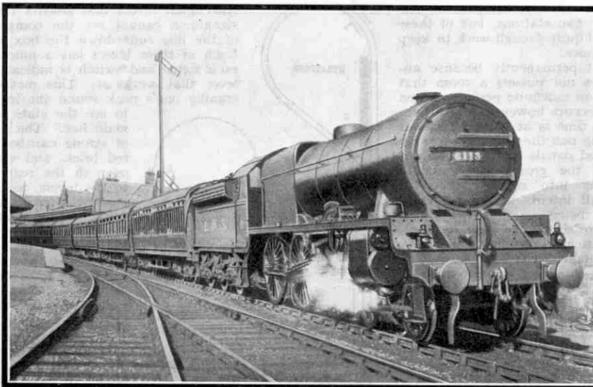
The "up" express leaving Penrith, hauled by L.M.S. "Royal Scot" type 4-6-0, No. 6113, "Cameronian." This is the locomotive that performed the record non-stop run on the "Royal Scot" train between London and Glasgow in April 1928
