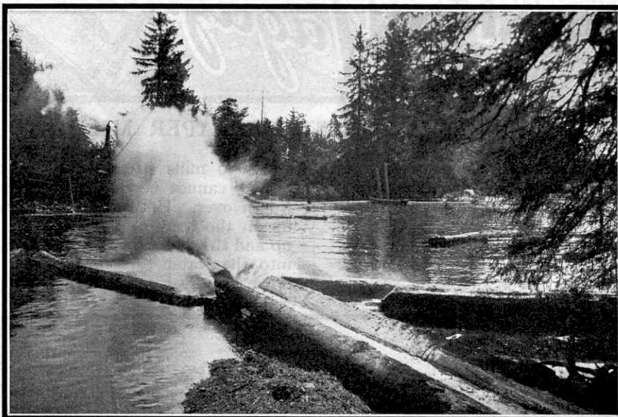
Chuting logs into a British Columbia waterway. The log that is entering the water has descended from the hillside forests in the flume seen in the foreground
