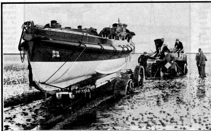
Launching a life-boat by means of a caterpillar tractor. This form of haulage has been found excellent where the boat has to be hauled across waterlogged sandy beaches. In the above photograph the depth to which the rear wheel of the boat carriage is sunk gives some idea of the difficulties involved
