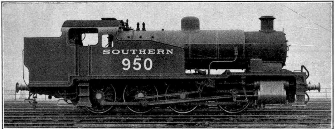
The first of a batch of eight new 0-8-0 shunting tank engines for service in the principal S.R. goods yards and sidings. We publish this illustration and the accompanying diagram by courtesy of the "Southern Railway Magazine"
