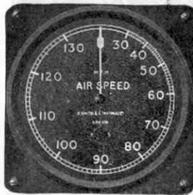
This dial shows air speed in miles per hour
