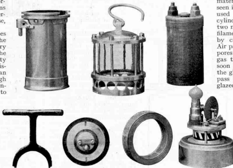
The parts of the Ringrose Fire-damp Alarm. In the upper row are the battery and the sections of the case, and on the right of the bottom row are the working parts of the Alarm. The porous cylinder may be seen below the lamp
