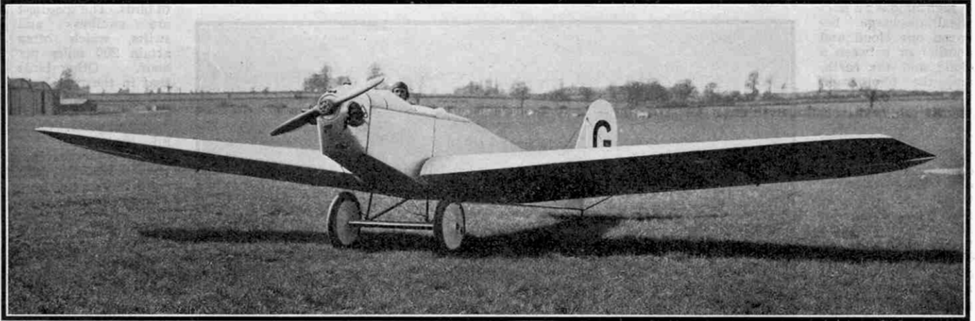
The Cherub-engined "Bristol" Brownie. For this and the other photographs illustrating this article we are indebted to the Bristol Aeroplane Co. Ltd., of Filton, Bristol
