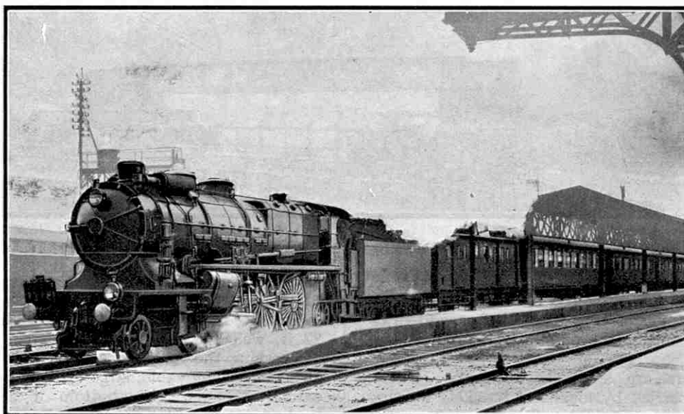
Nord "Pacific" No. 31225 at the head of the "Golden Arrow." The A.C.F.I. feed water heater fitted is carried on top of the boiler between the chimney and the steam dome.
