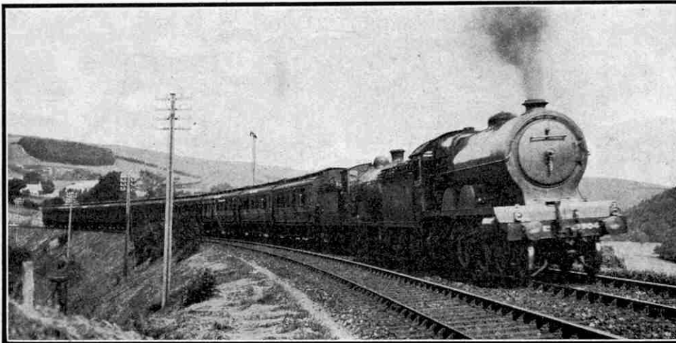
Double-heading on the steeply graded L.N.E.R. "Waverley" route between Edinburgh and Carlisle. The heavy express is hauled by 4-4-0 No. 9412, "Laird o' Monkbarns" piloted by a 4-4-2 No. 9904, "Holyrood."
