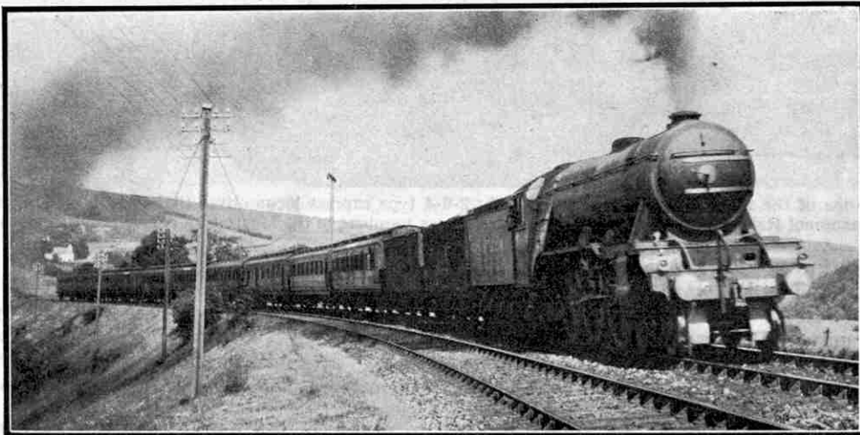
Pacific No. 2748, "Colorado" at the same point on the "Waverley" route as the train shown in the upper illustration on this page. This powerful locomotive is hauling with ease a load greater than that requiring two engines of older types.
