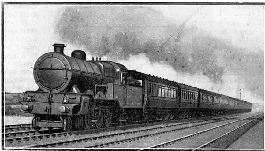
A Blackpool "Club" train at speed hauled by one of the Horwich-built 4-cylinder 4-6-0 type express locomotives of the L.M.S.
