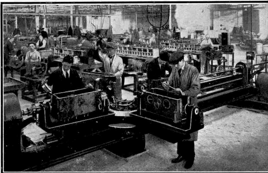
Reamering and crank fitting machine in the repair shop of the London General Omnibus Co.'s works at Chiswick.
