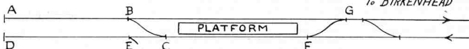
Diagram showing the operation of the automatic points system at Liverpool Central.
