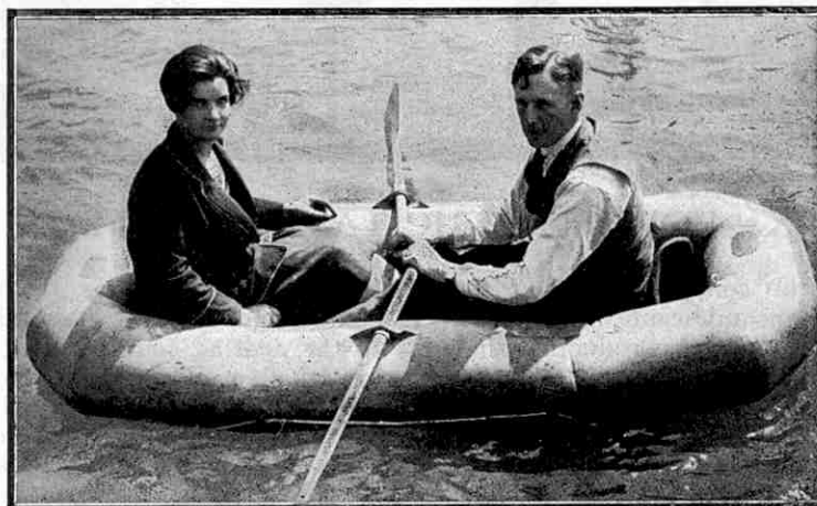
The folding air raft described on this page is large enough to accommodate two persons.
