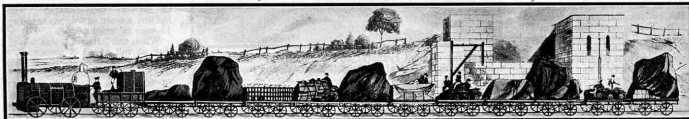
A goods train hauled by the locomotive " Liverpool " with its quaint-looking " haystack " firebox.
