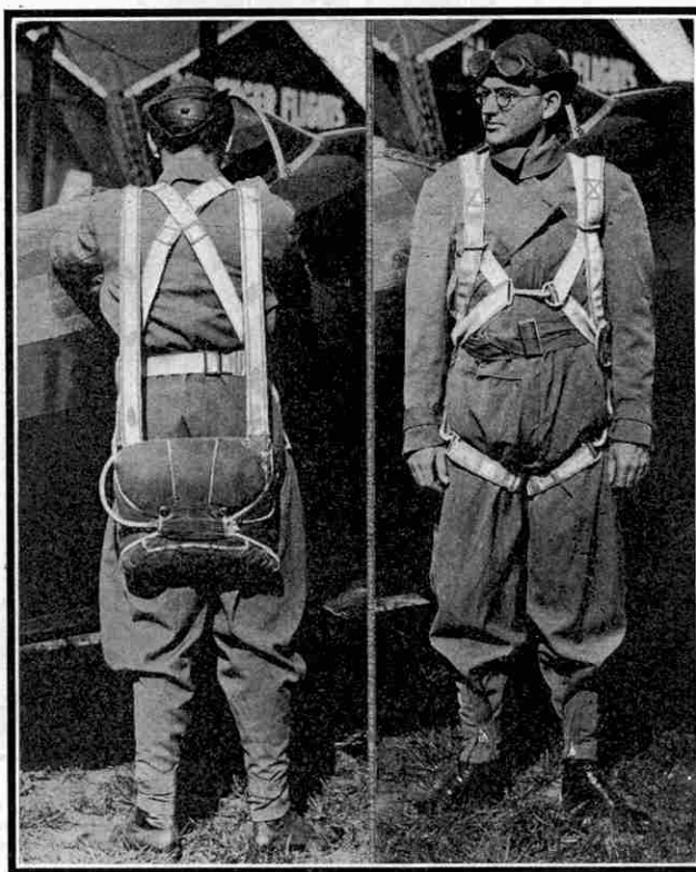
Photographs showing the harness by means of which the airman is suspended from the Irvin Air Chute. It is simply attached by means of three hooks. The sides of the pack spring open, and the parachute is released, when the ring on his left side is pulled.
