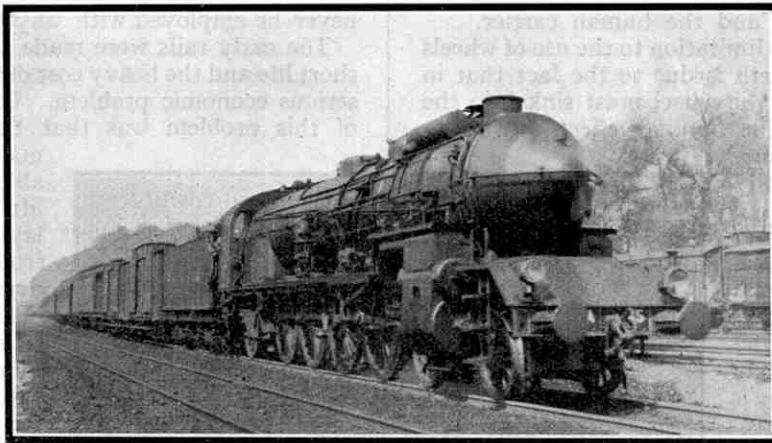
The P.L.M. No. 241-A-45 4-8-2 at Marseilles Rapide leaving Laroche. An engine of this type hauls the Blue train. For our photograph we are indebted to our reader, W. H. C. Kelland.
