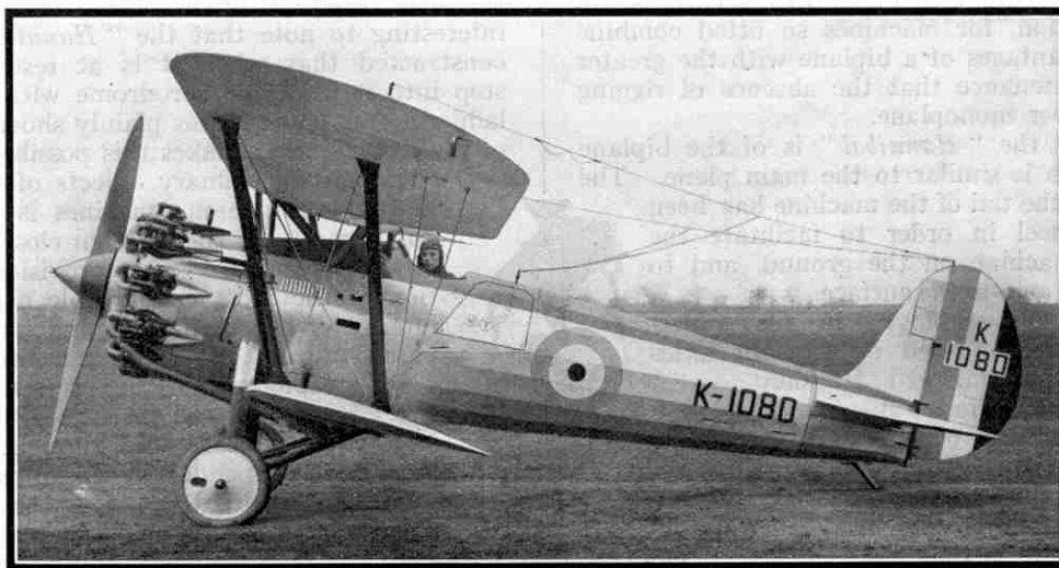
A side view of the Bristol "Bulldog" single-seater fighter machine, showing how the wireless aerial may be carried. We are indebted to the Bristol Aeroplane Co. Ltd. for permission to reproduce this photograph.
