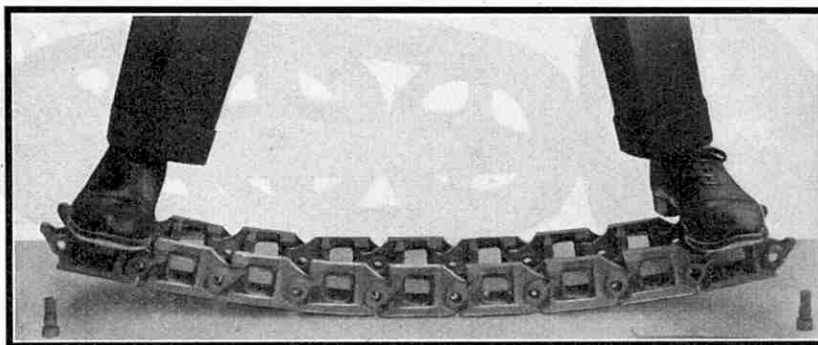
Man standing on "Orolo" links unconnected by pins, showing how these bear no stress from vertical loads.
