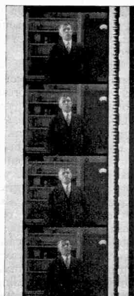
Variable width sound record on the right of film.
