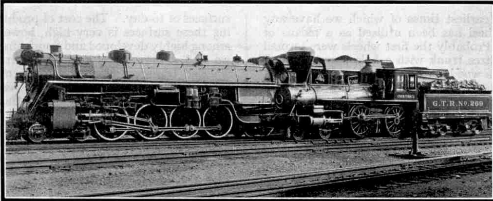
An early wood burning locomotive of the 4-4-0 or "American" pattern alongside a 4-8-4 locomotive of the C.N.R. "Confederation" type. Our photograph illustrates the growth of Canadian locomotives during the last 60 years.
