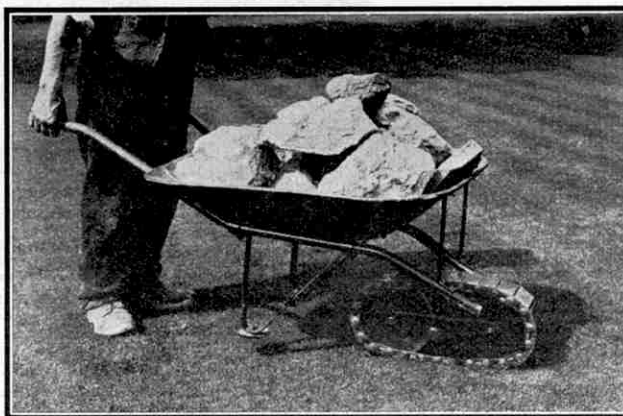
Barrow fitted with "Roadless" track unit in place of wheel.
