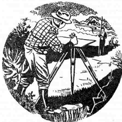
The engineer at work surveying virgin country with the use of a plane table. From "What Engineers Do" reviewed on this page.
