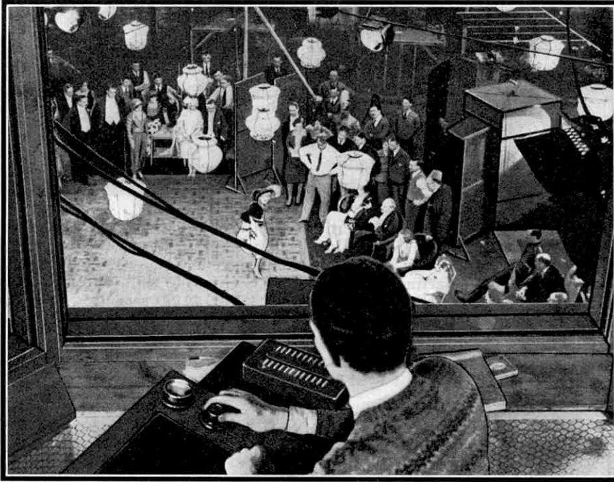
Looking down on the Sound Stage from the Monitor Room during the rehearsing of a set. The operator, or monitor man, is controlling the volume of sound passing from the stage to the sound recording room.
