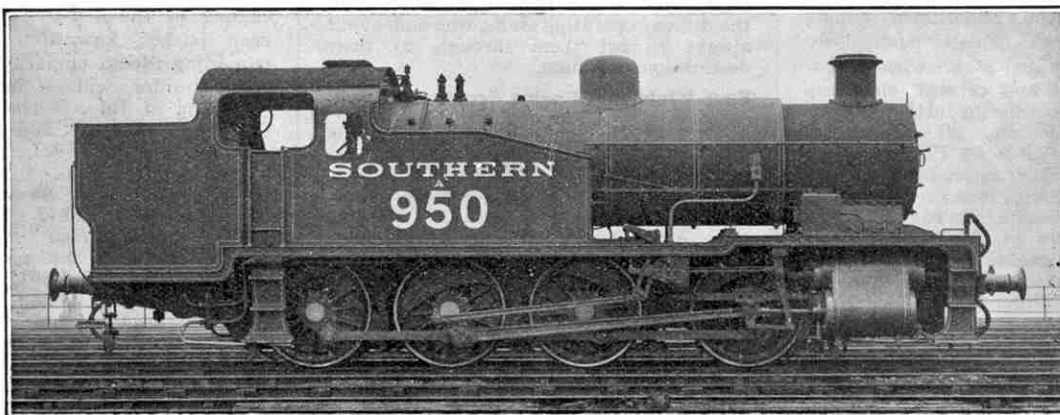
A three-cylinder 8-coupled tank engine specially designed for shunting work. Ample power is afforded by the cylinder and wheel arrangements adopted, and a moderate grate area avoids unnecessary fuel consumption when the engine is standing.
