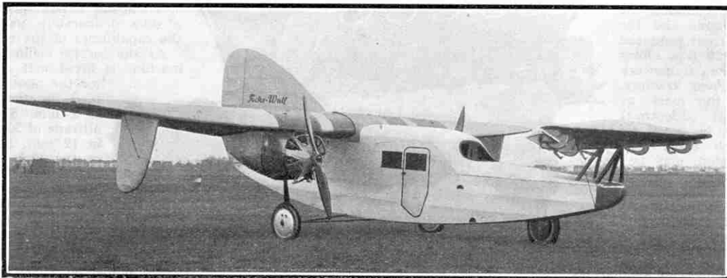
The Focke-Wulf "Ente," an interesting machine that flies with the main plane in the rear. For this photograph we are indebted to the Focke-Wulf Flugzeugbau A.G. The upper illustration on this page shows an early model of the Westland-Hill "Pterodactyl" and is reproduced by courtesy of the Westland Aircraft Works.
