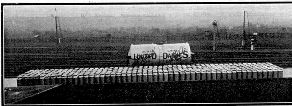
An interesting comparison showing the amazing economy in space afforded by the glass-lined milk tank wagons. The tank illustrated will hold as much as the 300 ten-gallon churns in the foreground.
