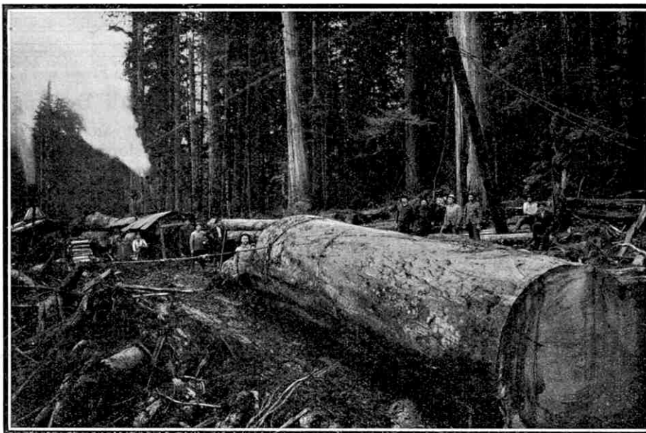
Dragging an 18 ft. sawn Columbian pine log by wire cables and donkey engine through timber wreckage to the logging train, for conveyance to the sawmill.
