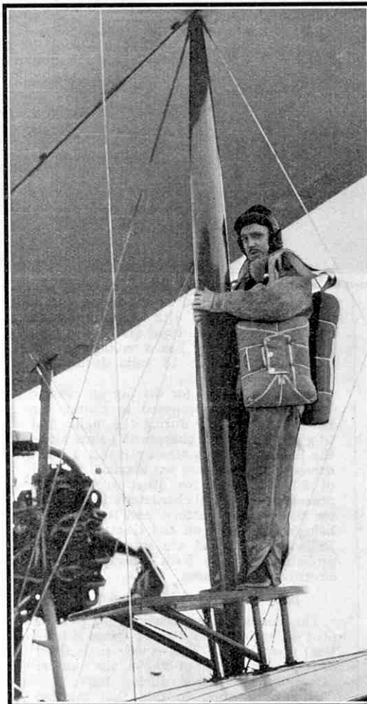
How a member of the R.A.F. makes his first parachute descent. Pulling the operating ring causes the parachute to open and he is pulled off the wing. The Vickers "Vimy" machines employed in training are fitted with wooden platforms for this purpose.
