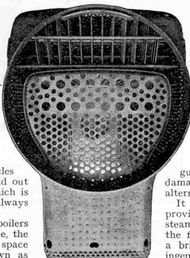
Interior of a boiler barrel showing the fire-box, tube-plate and stays.
