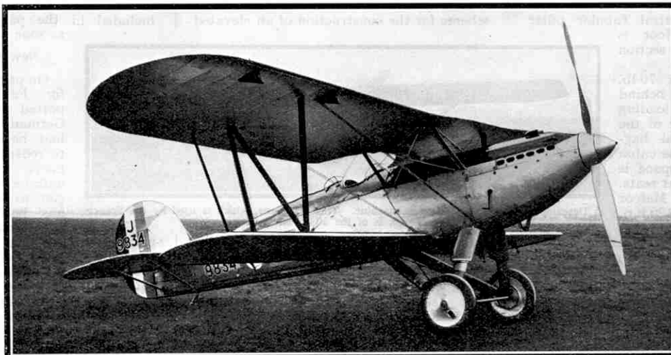
The Fairey "Fox II" day bomber equipped with a Rolls-Royce "Kestrel" engine. The racks on which the bombs are carried may be seen under the wings. Photograph by courtesy of the Fairey Aviation Co. Ltd.
