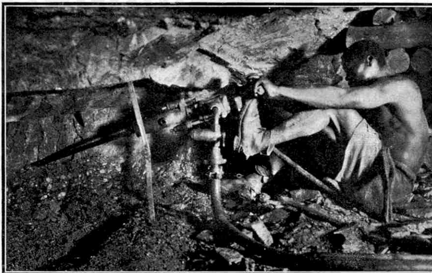
A native at work with a compressed air drill in one of the narrow levels of a South African gold mine. The photograph gives a good idea of the cramped quarters in which the miners work.
