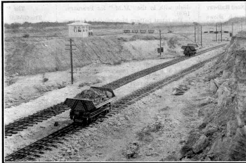
Motor-driven riderless cars on a remote controlled railway at Dallas, U.S.A. For our illustrations we are indebted to the General Electric Company, New York.
