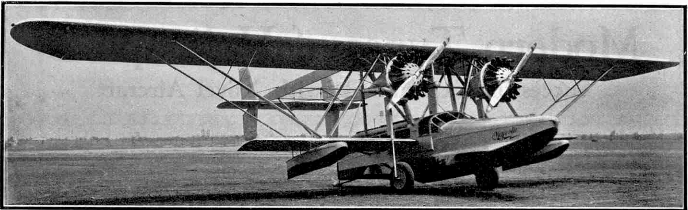
A Sikorsky amphibian. The two outriggers that support the tail unit of this interesting machine are plainly discernible. The total length of the flying boat is 40 ft. 3 in., while it measures 13 ft. 10 in. in height. Machines of this type are extensively used on American air lines.
