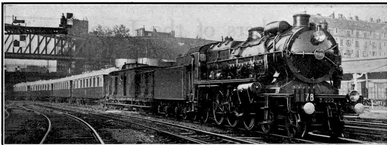
The "Golden Arrow" express on the Chemin de fer du Nord, headed by a compound locomotive of the "Pacific" type. The train number on the front of the engine is clearly seen. This number also is readily visible at night, when the figures are illuminated.
