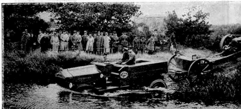
A Hathi Tractor hauling a heavy howitzer through a stream. (See next page).
