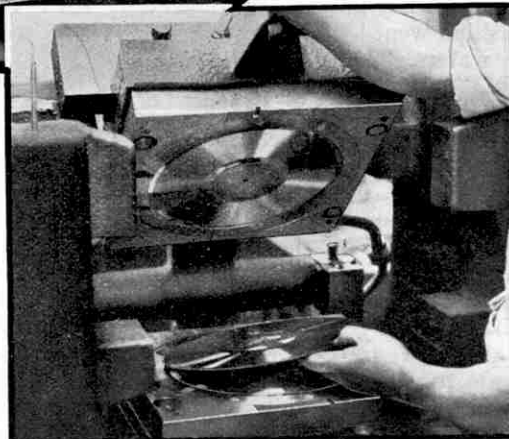
Pressing a "His Master's Voice" record. The material is rendered plastic on a hot plate (Above) and then placed on the matrix (Centre). The press is closed, pressure and cooling are applied automatically, and the press-man removes the finished record (Right). Photos by courtesy of the Gramophone Co. Ltd.
