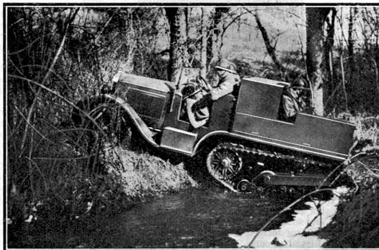
An armoured car equipped with creeper track fording a stream during military operations.
