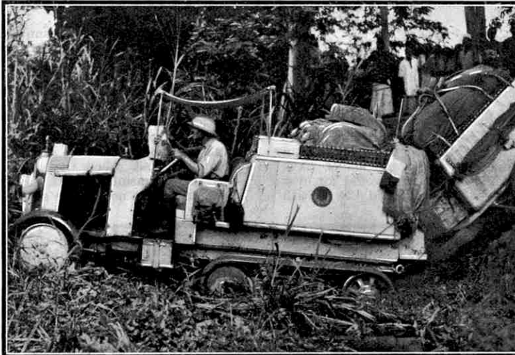
A Citroën Keggresse vehicle crossing a ditch during a long pioneer journey across Africa. The illustrations to this article are reproduced by courtesy of Citroën Keggresse Limited.
