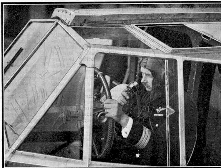
Mr. H. J. Horsey, a pilot of Imperial Airways, speaking into a Marconi microphone fitted in the cockpit of the Handley Page machine, "Hadrian." Our photograph is published by permission of Marconi's Wireless Telegraph Co. Ltd.
