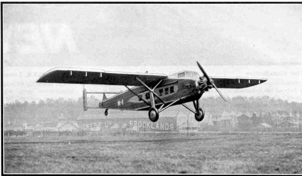
The single-engined version of the "Viastra" in flight over Brooklands Aerodrome. The machine illustrated is equipped with a Bristol "Jupiter X.F. BM" engine, but a wide choice of engines is available.
