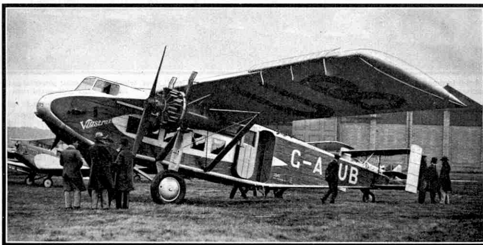
Three-quarter front view of the twin-engined Vickers "Viastra," showing the door open. The unusual rudders, described in the article, should be noted.
