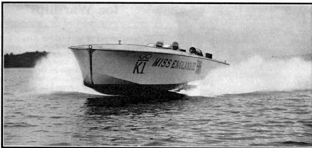
A splendid photograph of " Miss England III " at high speed. The stepped arrangement of the hull is well shown. For this and the photograph on the previous page we are indebted to J. I. Thornycroft Ltd.
