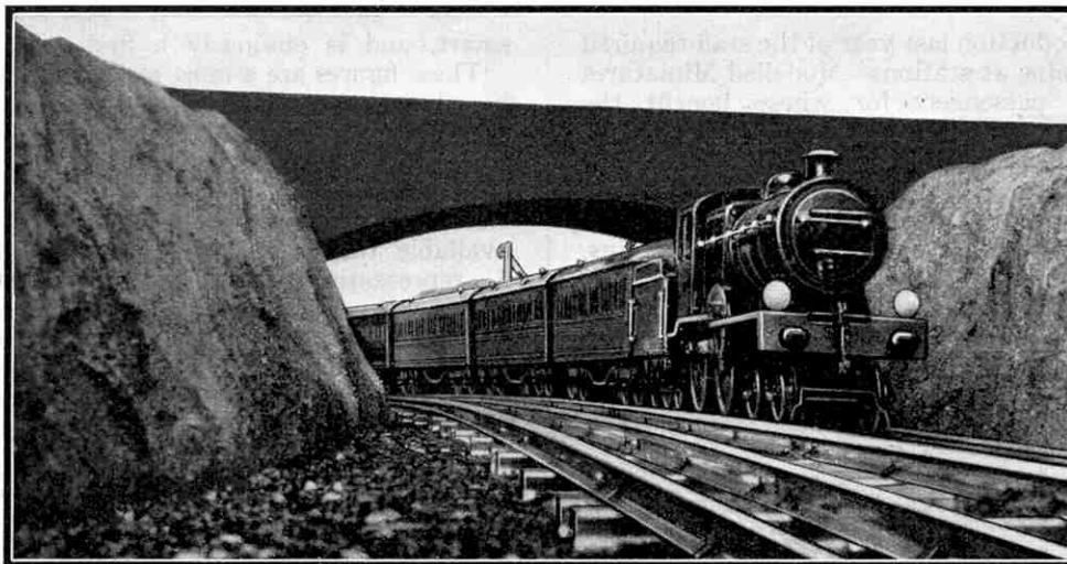
This photograph shows the use in miniature of discs instead of lamps as practised on the G.E. section of the L.N.E.R. They may be cut from white card and attached to the engines by means of suitable loops.
