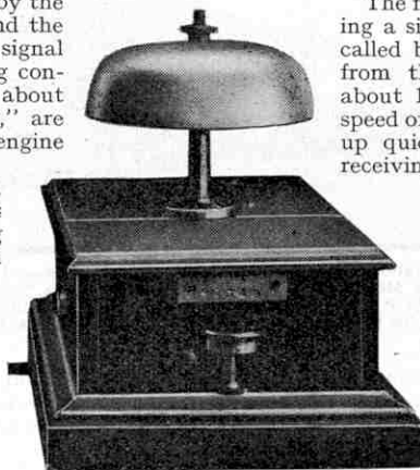
Tapper bell used by signalmen to communicate with each other by means of a code of rings.
