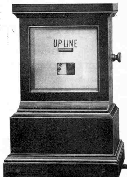
The smaller keyless instrument upon which the indication appears in the adjacent box.
