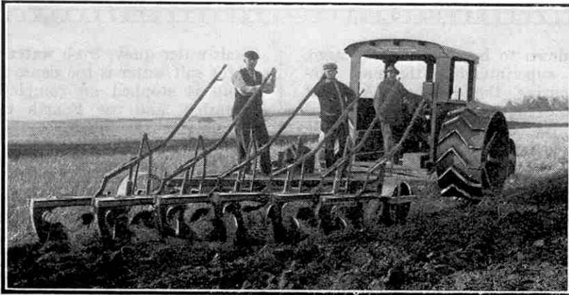
A modern multiple plough hauled by a large motor tractor. It is capable of doing six times the work of an ordinary horse plough.
