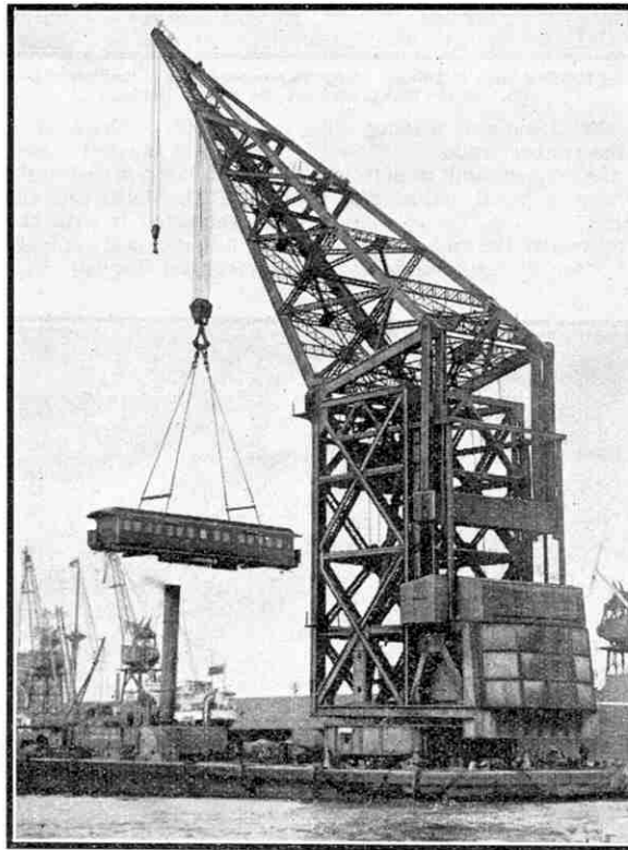
The 150-ton floating crane "London Mammoth" engaged on the shipment of railway coaches for South Africa. The illustrations to this article are reproduced by courtesy of the Port of London Authority.
