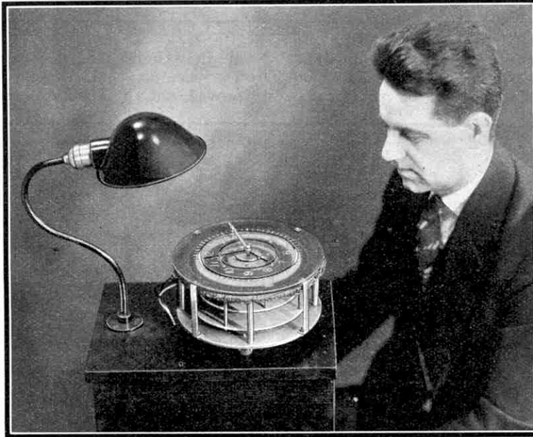
An electric clock that has no gear wheels. For our photograph we are indebted to the courtesy of the Westinghouse Electric Company.
