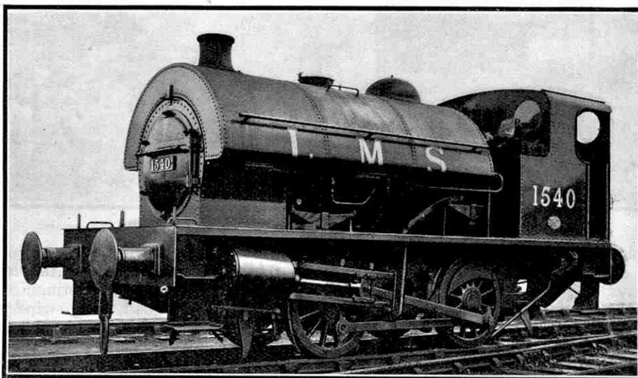
L.M.S.R. No. 1540, one of the new 0-4-0 saddle tank locomotives recently placed in service. The "stove-pipe" chimney is a new feature for engines of this line. Photograph by courtesy of the L.M.S.R.
