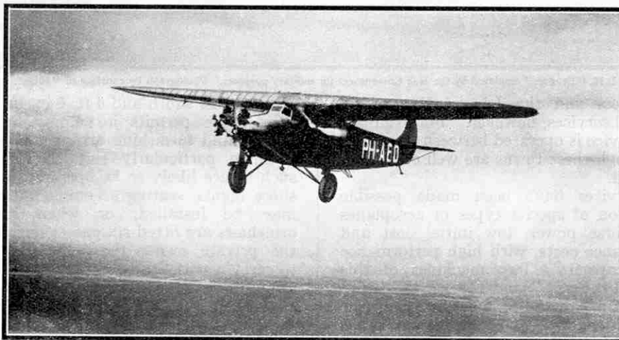
A Fokker F.VIIB—3m triple-engined high wing monoplane in operation on one of the air lines of K.L.M., or Royal Dutch Air Lines, to whom we are indebted for this illustration.
