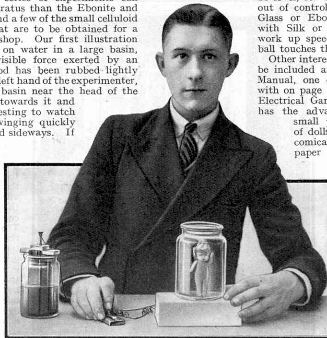
Fig. 1. A doll loaded with iron nails and immersed in water is caused to "dance" by means of an electro-magnet concealed in the stand.
