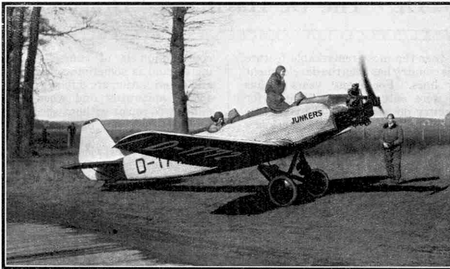
The start of a flight in the Junkers "Junior" light low wing monoplane. This machine was described on page 847 of our last month's issue. Photograph by courtesy of Junkers Flugzeugwerke, A.G.
