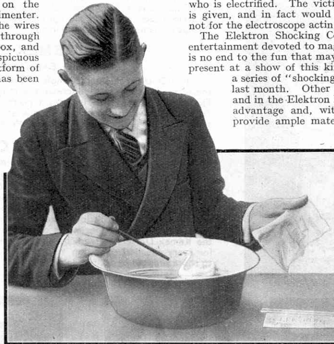
Fig. 3. Drawing a celluloid swan around a basin of water by the attraction of an electrified Ebonite Rod. An electrified Glass Rod produces the same effect.
