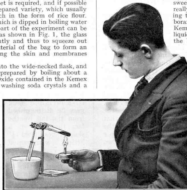
Fig. 3. Distilling a scented oil from dried cloves.
