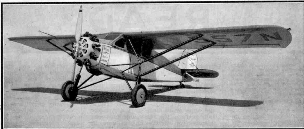
A three-quarter front view of an interesting American high wing monoplane, made by the Ryan Company. The machine illustrated is equipped with a Packard Diesel engine.
