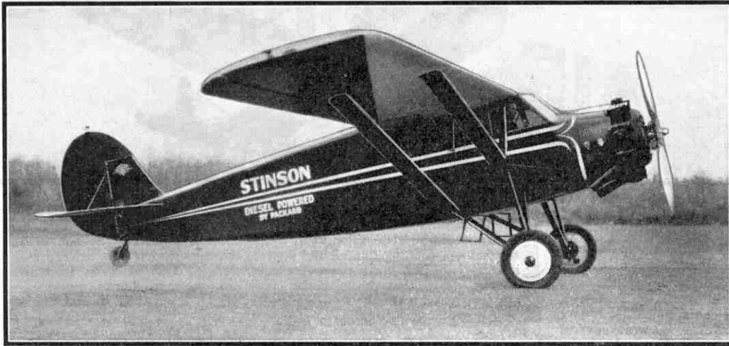
The Stinson "Detroit," the first American cabin machine to be provided with an engine starter and wheel brakes. The model illustrated is equipped with a Packard Diesel engine.
