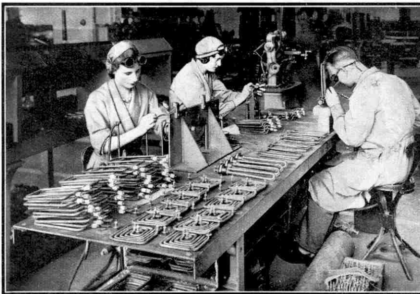
Fitting the terminals and ferrules to Torribar heating elements for use in electrical appliances.
