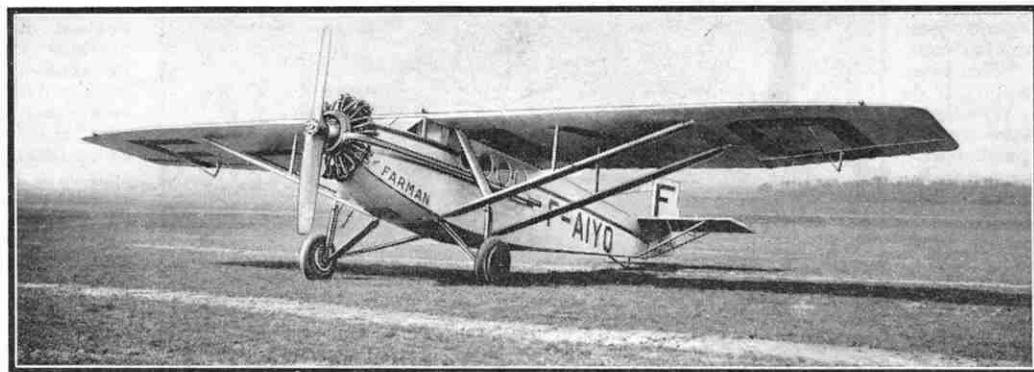
This photograph shows the Farman F-190 high-speed transport aeroplane, which has accommodation for four passengers and a pilot. Our photograph is published by courtesy of Avions Henri et Maurice Farman.
