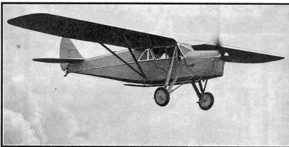
The D.H. "Puss Moth" light high wing cabin monoplane, which is being replaced by the "Leopard Moth," a slightly more powerful three-seater. Photograph by courtesy of the De Havilland Aircraft Co. Ltd.
