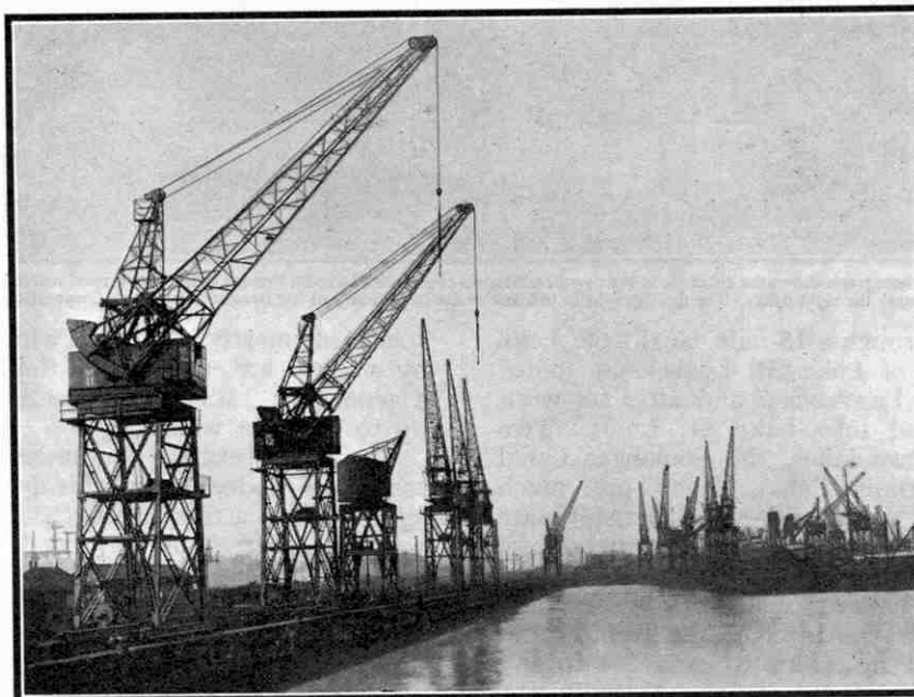
Level luffing cranes at Middlesbrough Docks. Photograph by courtesy of British Thomson-Houston Co. Ltd. See special article on page 275.
