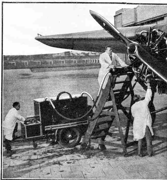
Philips "Metalix" X-ray equipment in use for testing part of an aero engine without removing it from the air liner in which it is fitted.
