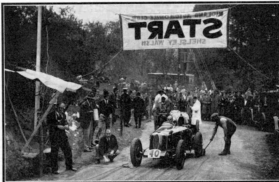
Starting a competitor in the Shelsley Walsh hill climbs organised by the Midland Automobile Club. The contact wire of the timing apparatus is in front of the off-side front wheel of the car. Another electrical contact is situated on the finishing line. Photograph by courtesy of the M.G. Car Co. Ltd.
