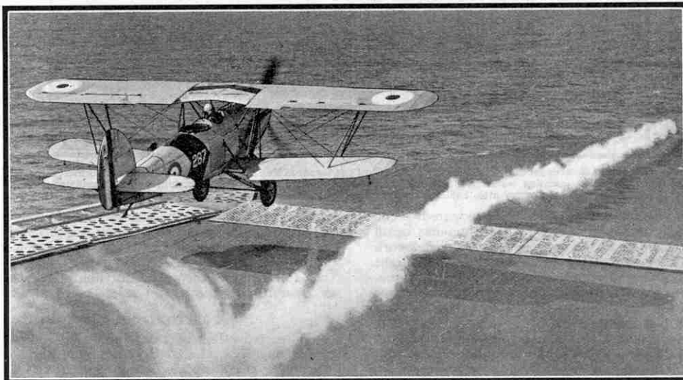
A two-seater Hawker "Osprey" taking off from H.M.S. "Eagle." The direction of the jet of steam shows that the carrier is steaming dead into the wind. Photograph by courtesy of "The Aeroplane."
