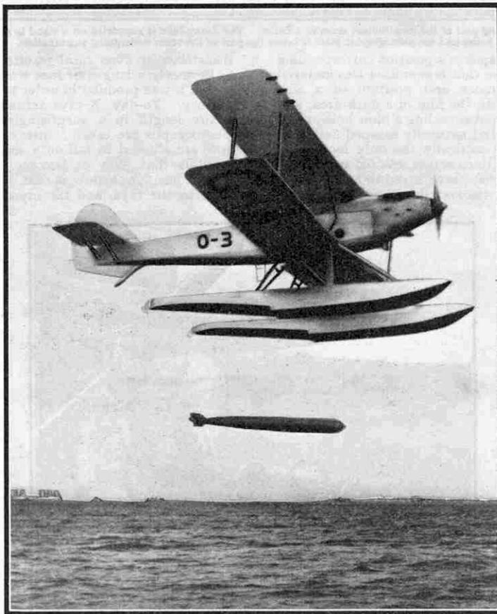
A Vickers "Vildebeeste" torpedoplane dropping a torpedo. Photograph by courtesy of Vicker's (Aviation) Ltd.
