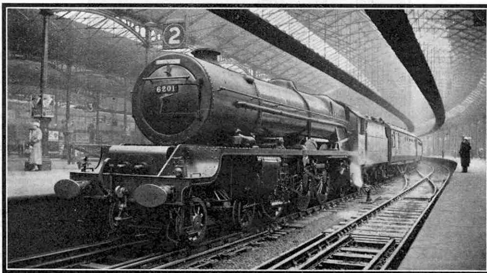
The upper photograph shows L.M.S.R. 4-6-2 locomotive No. 6200, "The Princess Royal." In the lower illustration is shown the second engine of this class to be constructed, No. 6201, "Princess Elizabeth," photographed on arrival at Euston. It bears the semaphore route indicator used on certain Scottish sections of the L.M.S.R.
