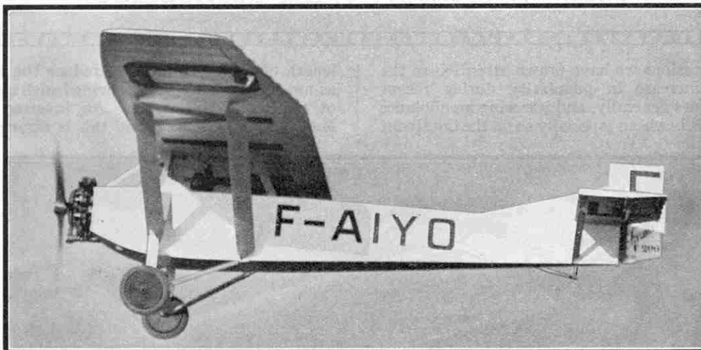
This photograph shows the Farman F.200, a popular French parasol monoplane that is equipped with a Salmson engine.
