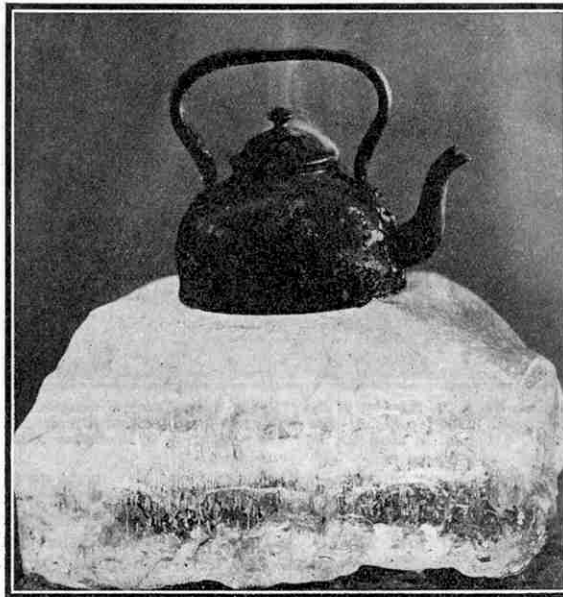
Boiling a kettle on ice. The kettle is filled with liquid air, which boils at a lower temperature than that of the ice. (From "Popular Scientific Recreations" reviewed on this page.)
