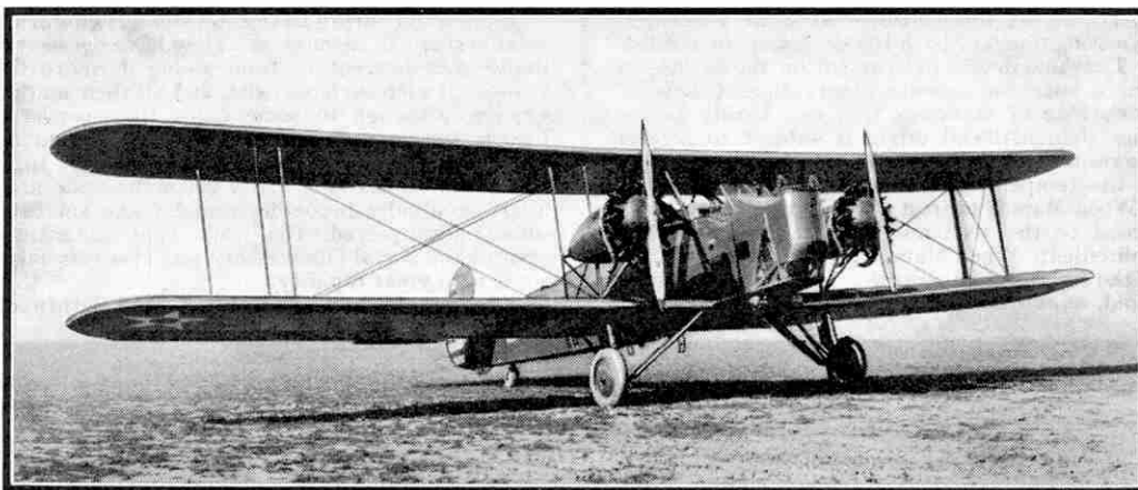
A Keystone bomber that forms the standard equipment of many of the United States Bombardment Squadrons. The latest version of this machine has a speed of 120 m.p.h. Official photograph, U.S. Army Air Corps.
