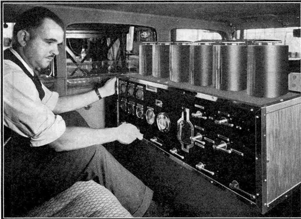
A motor car testing laboratory that can be installed in a few hours in any make of car in order to find the best grades of oil and petrol in various climatic conditions. We are indebted to the Associated Oil Company, California, for permission to reproduce this photograph.
