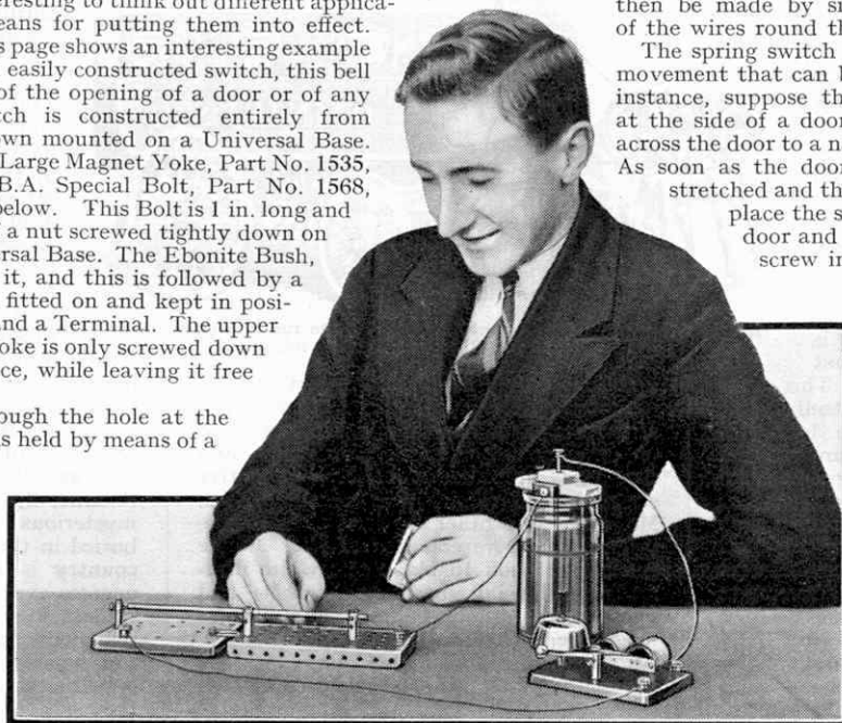
How a fire can be made to give its own alarm. The expansion of the rod when heated closes an electrical contact that causes a bell to ring.
