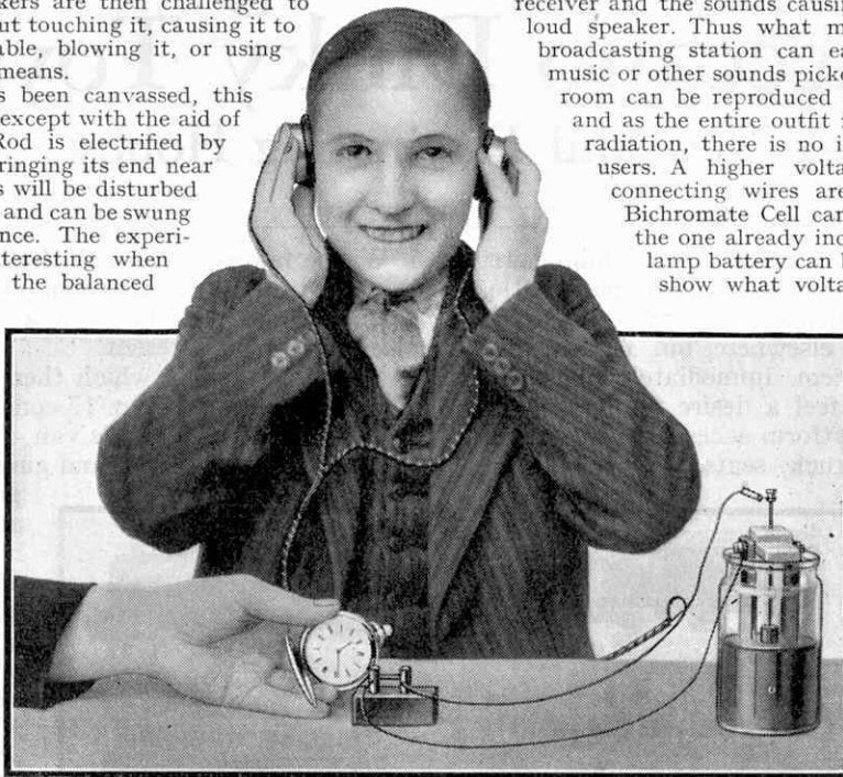
The ticking of a watch transmitted by means of a simple microphone and a pair of headphones.
