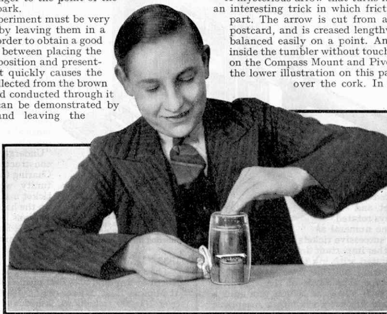
The magic arrow obediently turning towards the side of the tumbler covering it that is rubbed with a piece of silk.
