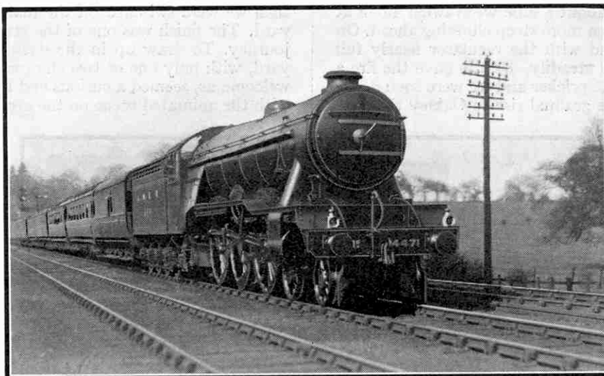
An L.N.E.R. up Harrogate express. The locomotive is No. 4471, "Sir Frederick Banbury," the second of the famous Gresley "Pacifics" to be built. Photograph by Real Photographs Co., Liverpool.
