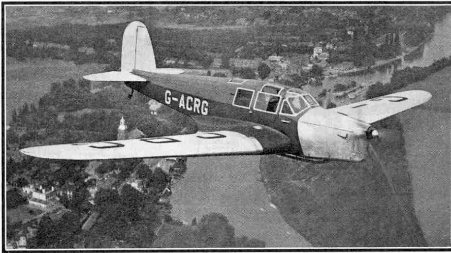
The British Klemm "Eagle" in flight over the Thames. The engine employed is a D.H. "Gipsy Six." For the photographs on this page we are indebted to the British Klemm Aeroplane Co. Ltd.
