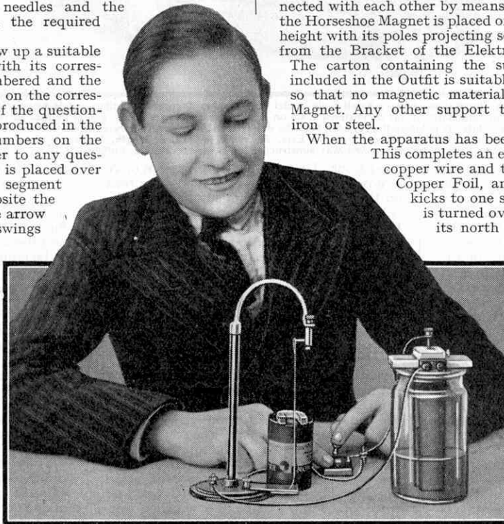
A vertical wire between the poles of an electro-magnet that swings to one side when current from the Elektron Bichromate Cell is passed through it.
