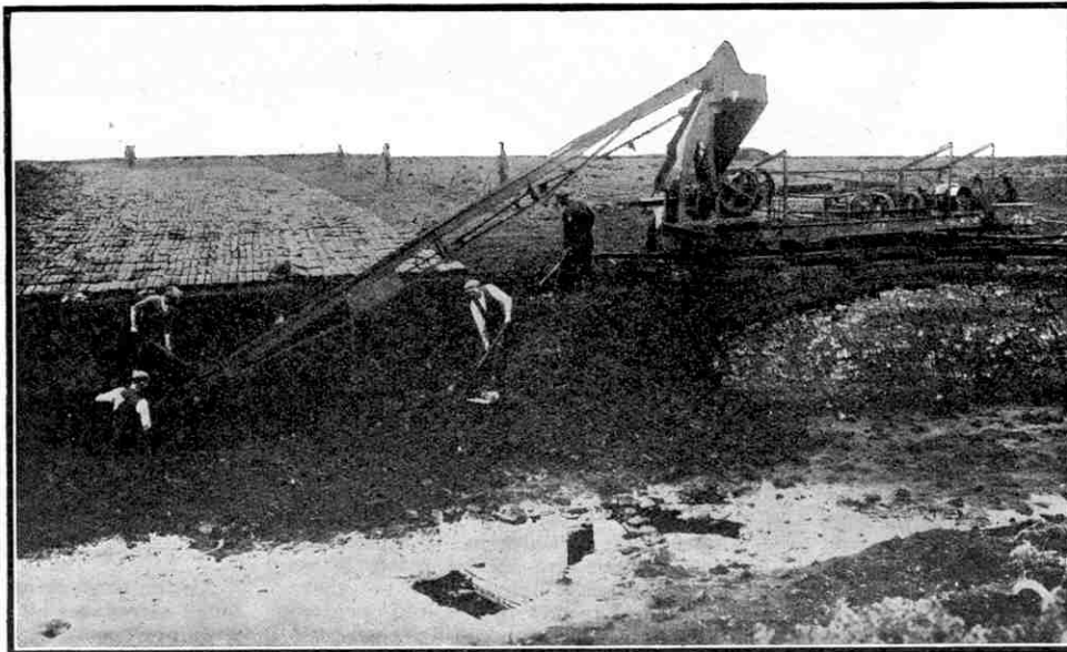
A semi-automatic macerator. The conveyor is hand fed and the peat is pressed into blocks of uniform size and shape.
