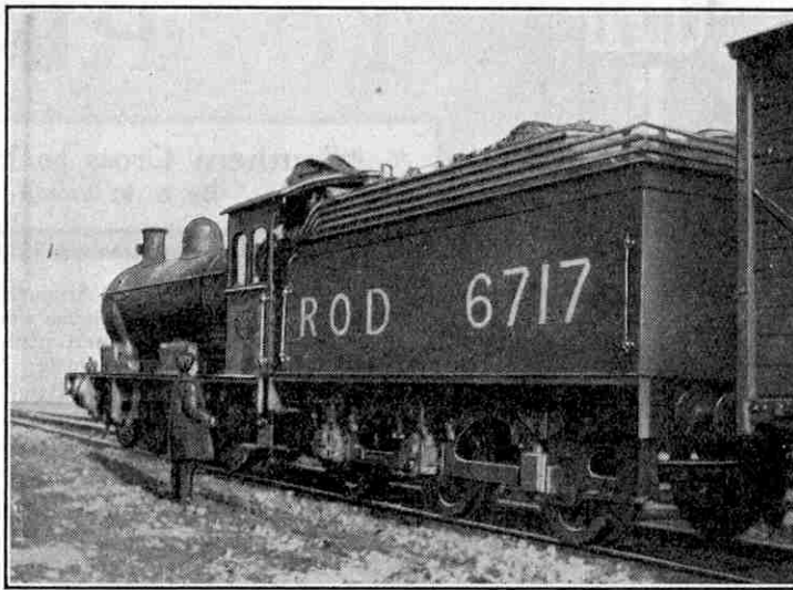
An 0-8-0 locomotive of the former North Eastern Railway photographed on active service. The lettering "R.O.D." on the tender signifies "Railway Operating Division."
