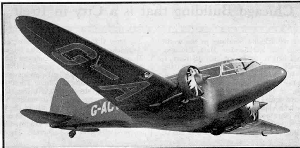
An impressive view of the Airspeed "Envoy," showing its similarity to the single-engined "Courier." The machine cruises at 150 m.p.h. and lands at 61 m.p.h. Photograph by courtesy of Airspeed Ltd.
