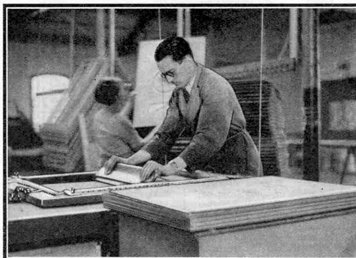
This illustration shows a silk screen operator squeegeeing a print. By a steady sweeping movement of the rubber squeegee the operator presses the paint through the silk screen, which is held taut in the oblong frame on the printing bench.
