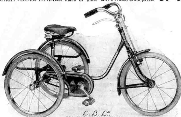
"TRI-ANG UNITY" JUVENILE CYCLE No. 9 (BOY'S) Frame of best quality weldless steel cycle tubing. Adjustable ball bearings throughout. 16 in. x 1 1/8 in. Dunlop pneumatic tyres on rustless tangent spoked wheels. Two rim brakes. Raised Handlebars. 1/2 in. x 1/4 in. cycle roller chain. Three coil saddle. CHROMIUM PLATED FITTINGS. Black or blue. Girl's Model same price. 57/6
