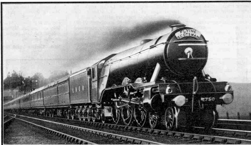
The L.N.E.R. "Super-Pacific" locomotive No. 2750, "Papyrus," that was used on the record-breaking runs described on this page. It is here shown in ordinary service on the down "Flying Scotsman" express. Photograph by Real Photographs Co., Liverpool.
