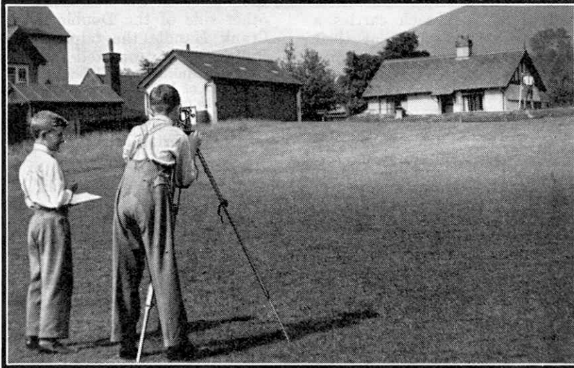
Mapping a field with the aid of a Meccano theodolite. The instrument is being sighted on the staff held upright on the edge of the field.
