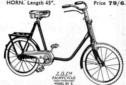
FAIRYCYCLE (Regd. Trade Mark) No. 2. Tubular frame, best quality British steel. Tangent spoke wheels. 1 1/2" imitation pneumatic tyres. Raised handlebars. Coil-spring saddle. Chain cover carrier. Rim brake and ball-bearing pedals. Black or blue. CHROMIUM-PLATED FITTINGS. Price 39/6.
