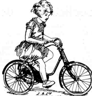
TRI-ANG TRICYCLE No. 5. (Regd. Trade Mark.) Now fitted with rear mudguards. Cycle chain drive with free wheel. Frame best quality weld-less cycle tubing. 14" wheels. 1 1/2" jointless sponge rubber tyres. Rim brake. Coil-spring saddle. CHROMIUM FITTINGS. Black or blue. Price 59/6.
