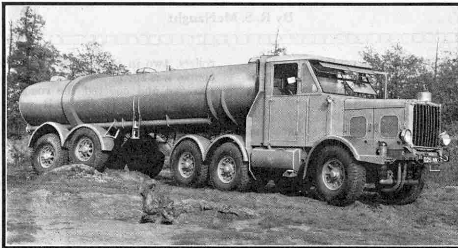
A giant 10-wheeler Scammell Oil Tanker capable of carrying 4,200 gallons of oil fuel. It is one of two similar vehicles built for service overseas, and is equipped to traverse rough country should occasion arise. Photograph by courtesy of Scammell Lorries Ltd., London.
