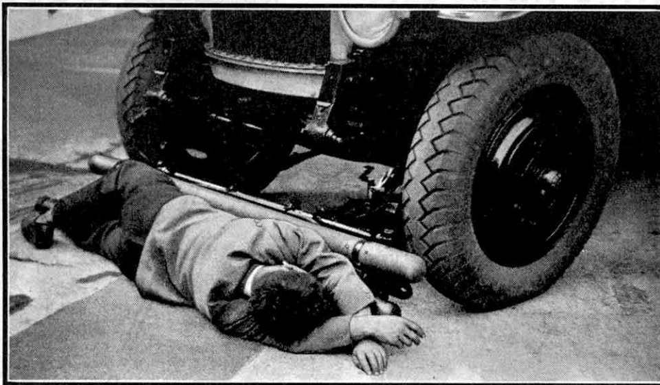
The "Safety Bumper" rolling a man along the ground after he has thrown himself in front of a 3-ton truck. Photograph by courtesy of Safety Bumpers Ltd., London.
