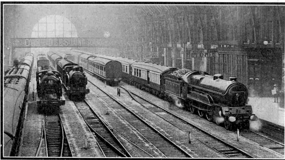
An interior view of part of King's Cross station. At the main departure platform is one of the Great Central 4-cylinder 4-6-0 engines at the head of the "Harrogate and Edinburgh Pullman" train, as the "Queen of Scots" was formerly known.
